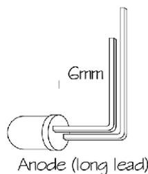
Bend the leads of D10 right angle at 6mm from the body taking care of the anode position (the longest lead). Insert from the PCB B side and solder with the leads at 2mm from the PCB surface.
