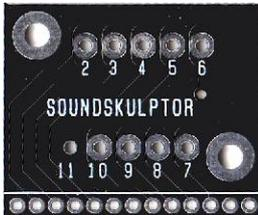
Use the input transformer front PCB, the one with the pin holes and numbers. Two units of this PCB are available. Only one will be used. Insert the 90°, 13 pins headers, long tails first, into the holes, from the top side, marked SOUNDSKULPTOR.
