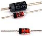
Add D1, D2, D5. Use a lead forming tool to bend the leads at 0.4".
