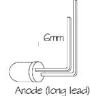
Bend the leads of D I O right angle at Gmm from the body taking care of the anode position (the longest lead). Insert from the PCB B side and solder with the leads at 2mm from the PCB surface.
