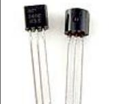
Add Q1. It must be placed flat on the PCB, flat side against PCB.
