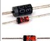
Add D5 to D9. Use a lead forming tool to bend the leads at 0.4".
