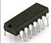
Insert U3 and solder. You will need to bend the pins slightly inwards before inserting. Make sure you are not charged with electrostatic electricity before handling the IC (or remove your shoes).
