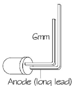
Bend the leads of D5 right angle at 6mm from the body taking care of the anode position (the longest lead). Insert from the PCB B side and solder with the leads at 2mm from the PCB surface.
