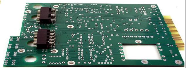
Warning: The connectors are installed on the solder side of the PCB.
